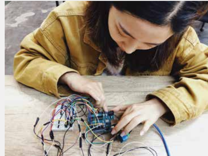
STEP 4: Connect all the wires with breadboard and Arduino board.
