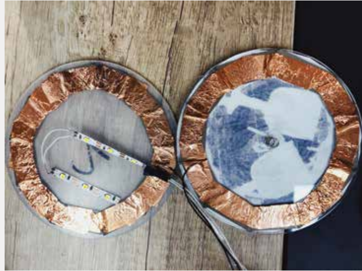
STEP 1: Cut out the cup-holders, attach them with LED strips, and solder the wires and springs to make it a button.
